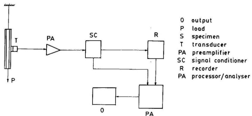
The electrical signals received by an AE sensor are processed by a wide variety of parameters
