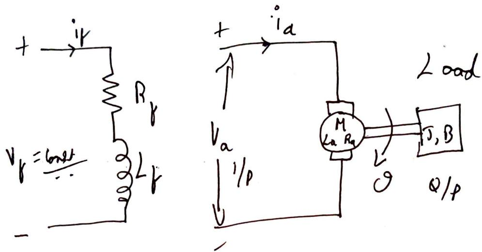
Let,  $R_a$   $\rightarrow$  Armature resistance,  $\Omega$  $L_a$   $\rightarrow$  " " Inductance,  $H$  $i_a$   $\rightarrow$  " " current,  $A$  $V_a$   $\rightarrow$  " " Voltage,  $V$  $e_b$   $\rightarrow$  Back emf,  $V$  $K_t$   $\rightarrow$  Torque constant,  $N-m/A$  $K_b$   $\rightarrow$  Back emf constant,  $V/(rad/sec)$
