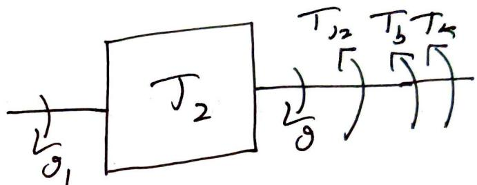
$$T_2 \frac{d^2 \vartheta}{dr^2} + \beta \frac{d \vartheta}{dt} + k(\vartheta_2 - \vartheta_1) = 0$$
