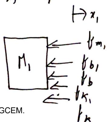
$$f_{m_1} = M_1 \frac{d^2 x_1}{dt^2}; \quad f_{b_1} = B_1 \frac{dx_1}{dt}; \quad f_{k_1} = k_1 x_1$$
