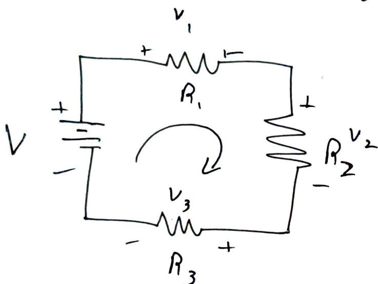
$$V = V_1 + V_2 + V_3$$
