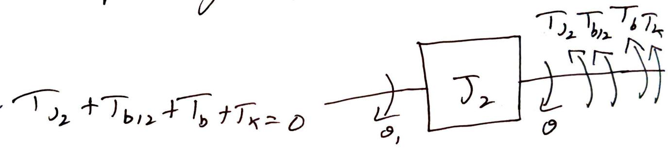
$$\bar{T}_{J2} + \bar{T}_{b12} + \bar{T}_b + \bar{T}_k = 0$$
