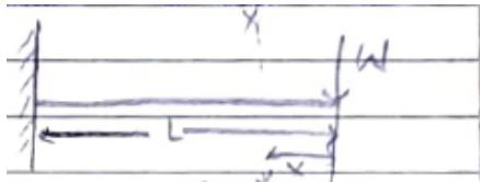
Fig 8 shows a cantilever beam of length  $L$  subjected to point load at the free end.
