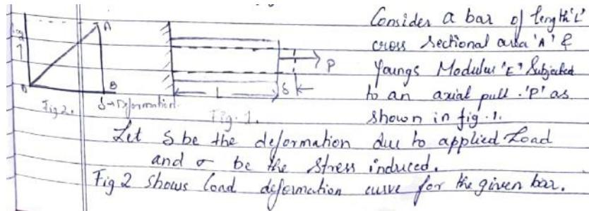
Work done by the applied load is equal (Work done) to area of triangle  $AOB$
