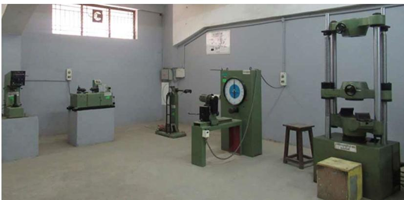
The Aeronautical department is well equipped & technically organized Laboratory for the Material testing and metallurgy Laboratory. Testing of materials for their mechanical properties forms an integral part of this lab. In this lab the students conduct experiments on Universal testing machine, various hardness testing machines, Wear, Impact, fatigue and Torsion testing machines.
