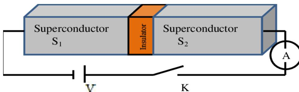
Because of the DC voltage applied across the barrier, the energy difference of cooper pairs on both sides is of the order of 2eV.
